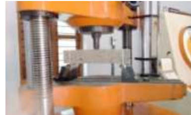
Fig 7. Flexural strength checking
